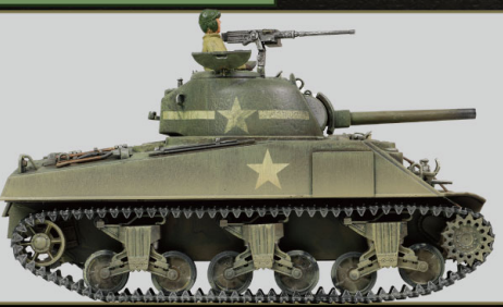
The later version having a "sharp-nose" style. The upper border, along the bolt strip, also evolved, so that the bolts were better protected against shells and explosive devices.
