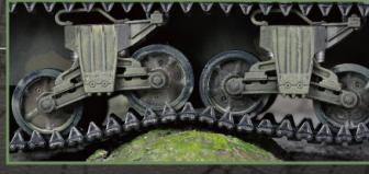
Bogie assembly, Vertical volute spring, with the "offset roller" and skid. The most common type that can be found on Sherman tanks.
