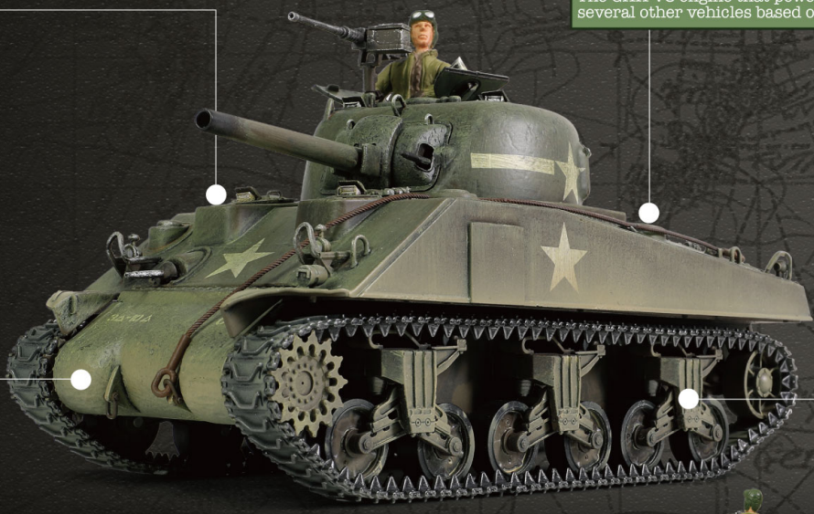
The drivers' hoods were redesigned to eliminate them. The hoods were elongated in the front, where an additional periscope was provided.
