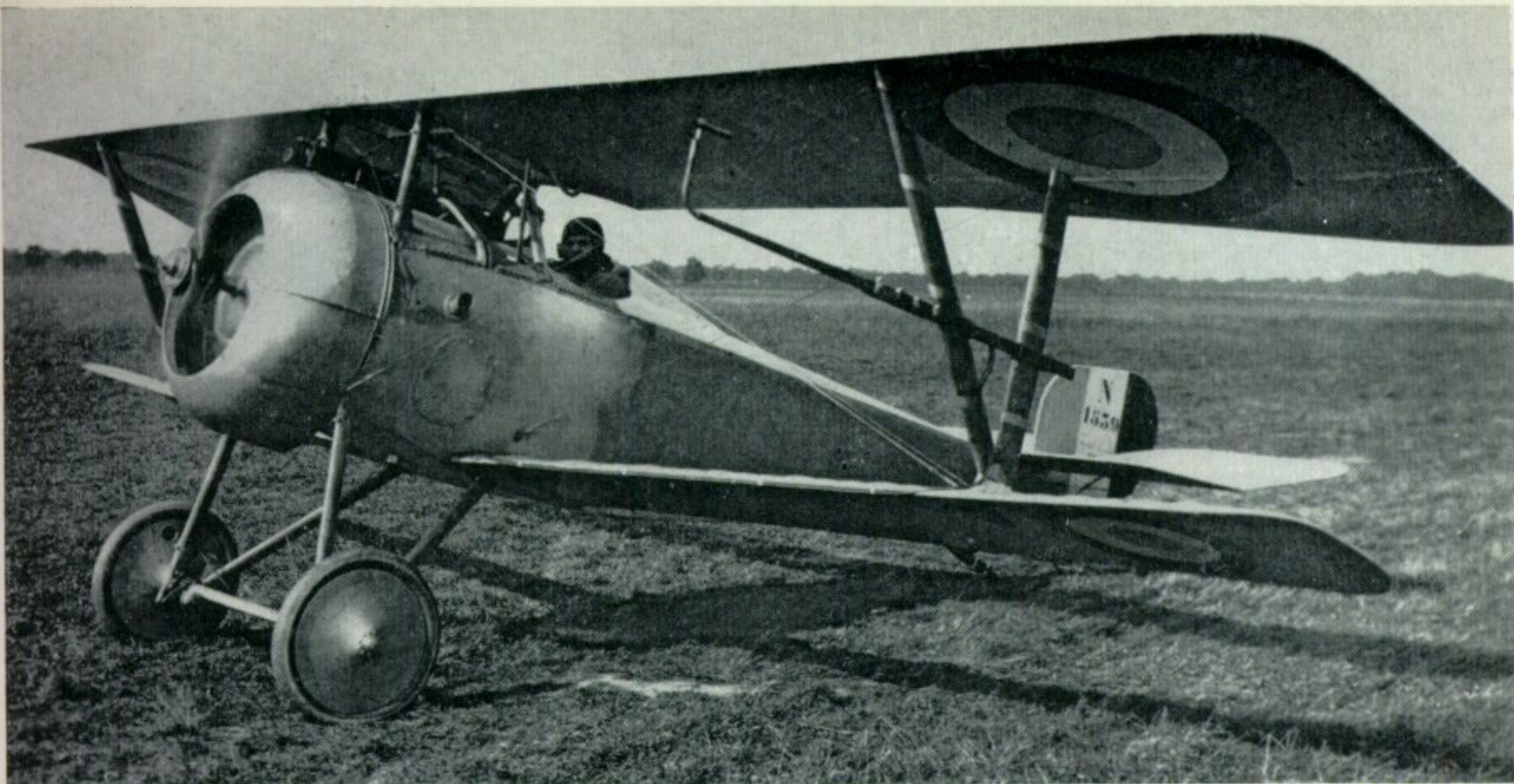
A French Nieuport 17 with fuselage-mounted Vickers gun and experimental pitot "yawmeter". (Photo: Imperial War Museum)
