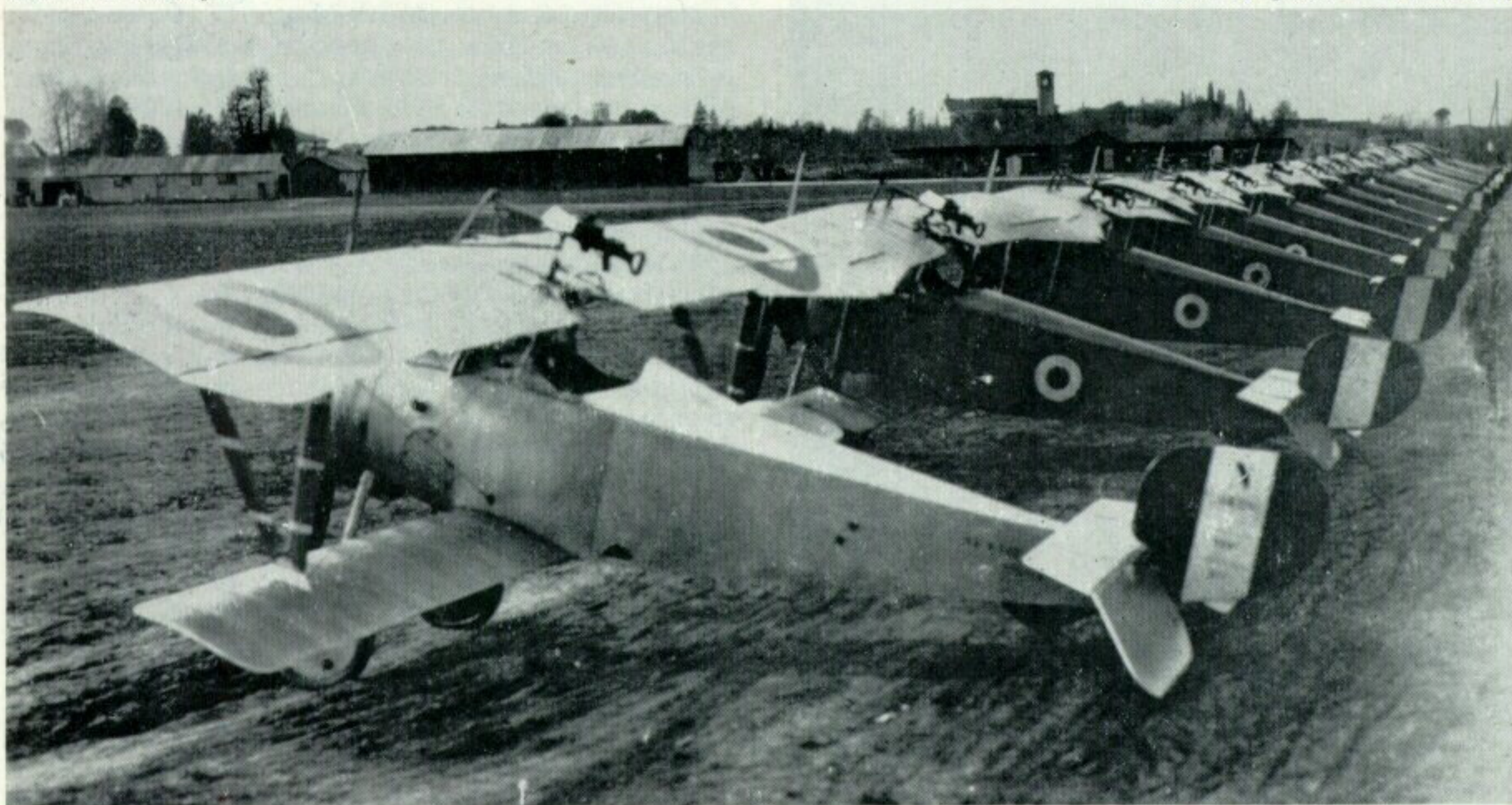
A line-up of Italian Nieuports in 1917 of Types 11 (Bébé) and 17. The latter may be distinguished by the pilot's head fairing, as on the nearest aircraft. (Photo: Imperial War Museum)
