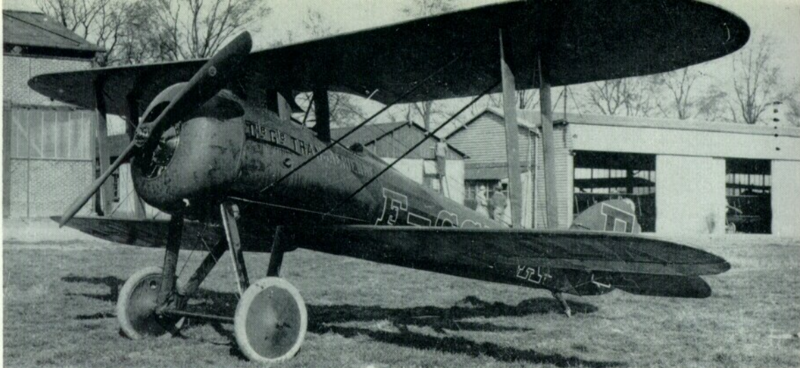
A post-war civilian conversion with an 80-h.p. Le Rhône engine. Although carrying French registration, this must have been an A.E.F. left-over because the "Lift Here" placards on the fuselage are in English. (Photo: SAFARA)
