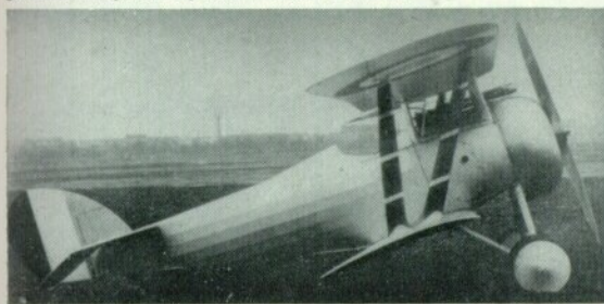
Left: Further evolution of the Model 28—a modified 24 with enlarged two-spar lower wing that increased the total wing area to eighteen square metres from the fifteen of the standard Model 24. Right: Original prototype of the Nieuport 28 with single machine gun and unique one-piece interplane struts. (Photos: Nieuport)
