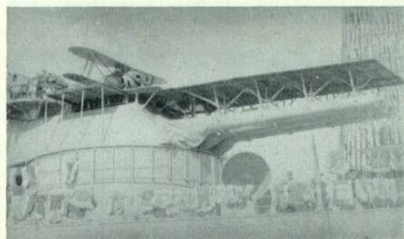
Left: U.S. Navy Nieuport 28 on gun turret of the battleship Arizona. Such use of airplanes, tried by French and British as well as U.S. Navies, was short-lived. Right: Top view of silver-painted Nieuport 28 on battleship Arizona. The original wartime roundels show through the post-war star-in-circle markings on the wings. Tail stripes on this particular model are still in the original Nieuport width. (Photos: U.S. Navy)
