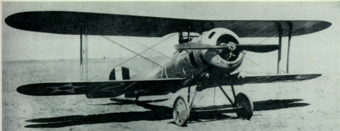
U.S. Navy Nieuport 28 with flotation gear, star insignia, and reduced-size tail stripes.
