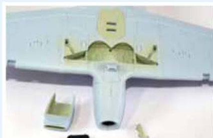
Photo 8 Oil Coolers intakes and radiators are fitted to the underside of the wing while a small pipe is fitted in the centre of the undercarriage bay.
