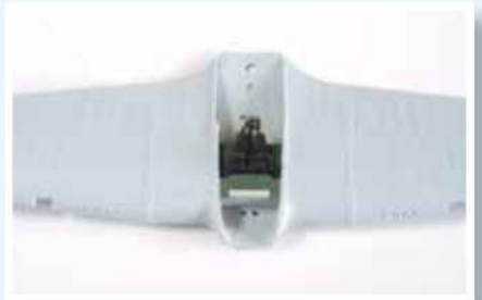
Photo 6 The cockpit floor, rudder pedals and control column assembly is cemented to the upper wing spar.
