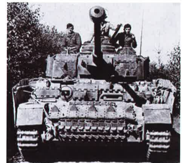
panzer IV mounted with soviet t-34's tracks
